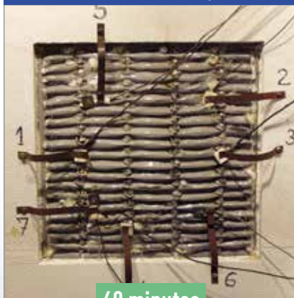
VENTILODICE V after 60 minutes of the fire resistance test (non-exposed side)
